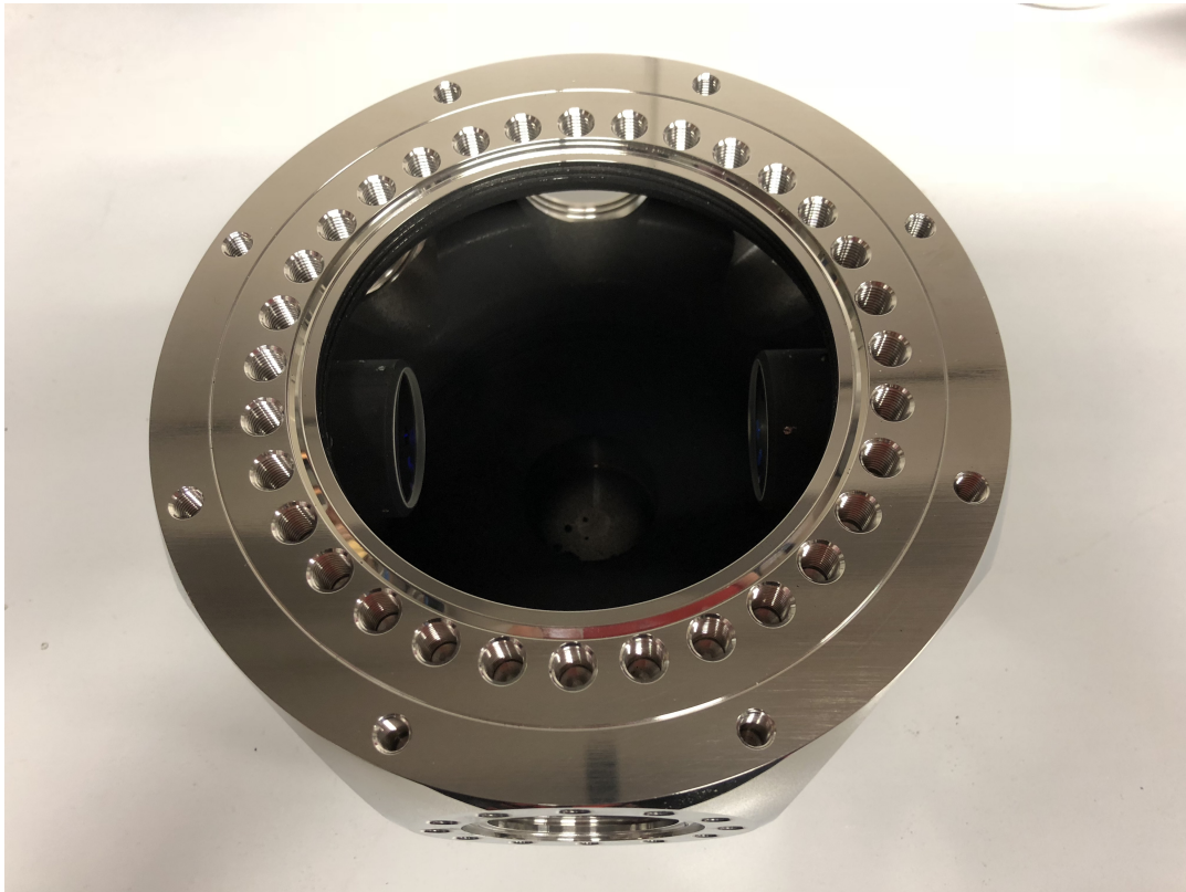
FIGURE 4.25: Coating of the magneto-optical trap and detection optics. The blank stainless-steel surfaces on the inside of the vacuum chamber have been coated with a black paint (AZ Technology MLS-85-SB-C) to reduce stray light. The coating was developed for the use in the Low Earth Orbit space environments and has a low out-gassing rate, therefore suitable for the ultra-high vacuum environment in the magneto-optical trap. The aluminum lens holder tubes have been coated on the outer and inner side. The anti-reflective coated lenses are chosen as large as possible to maximize the numerical aperture and therefore the signal of single atoms.
